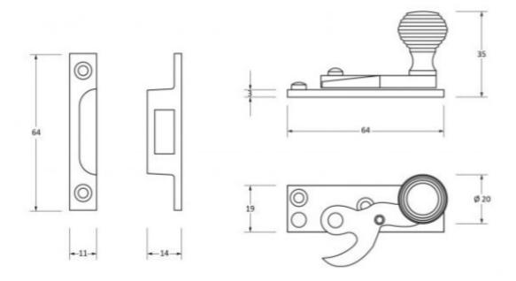
• Fixing plate: 64mm x 19mm
