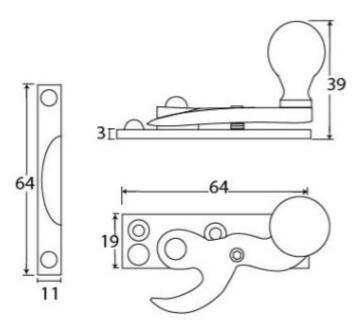
• Fixing plate: 64mm x 19mm
