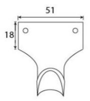
• Fixing plate: 51mm x 18mm
