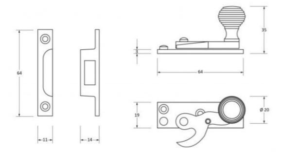
• Fixing plate: 64mm x 19mm
