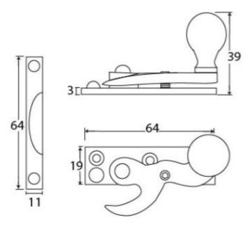
• Fixing plate: 64mm x 19mm
