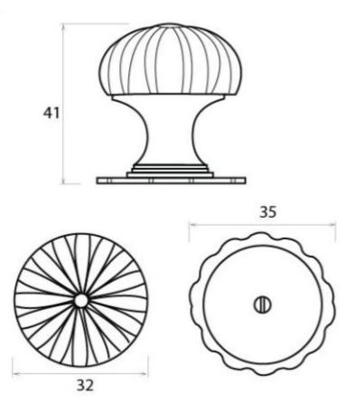
Overall Size: 32mm DiameterBase Size: 35mm DiameterProjection: 41mm
