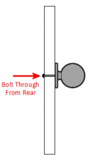
• Bolt through fixings provide a superior strong fixing allowing this knob to be fitted to tall or heavy doors
