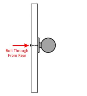
• Bolt through fixings provide a superior strong fixing allowing this knob to be fitted to tall or heavy doors
