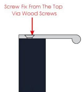
• Supplied with matching countersunk slotted wood screws
