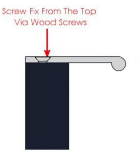
• Supplied with matching countersunk slotted wood screws
