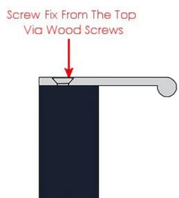
• Supplied with mPCching countersunk slotted wood screws
