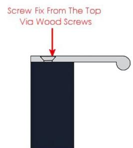
• Supplied with mSNching countersunk slotted wood screws
