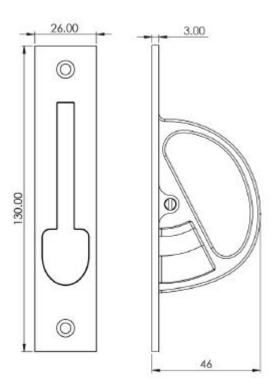
Plate Size: 130mm x 26mmFaceplate thickness: 3mm
