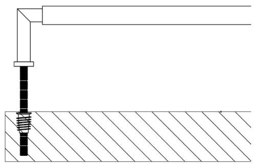
Above diagram shows how a face fix pull handle is fitted to a wooden door
