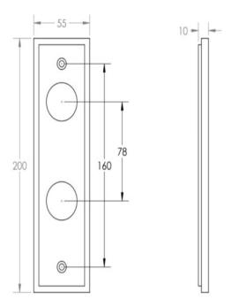
• DIN Bathroom Lever Set - 78mm Centres - (With Turn & Emergency Release)
