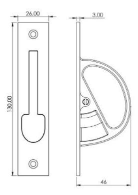
Plate Size: 130mm x 26mmFaceplate thickness: 3mm
