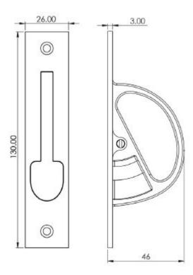
Plate Size: 130mm x 26mmFaceplate thickness: 3mm
