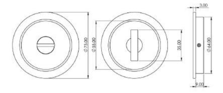
• Turn & Release - 75mm Diameter x 12mm depth.
