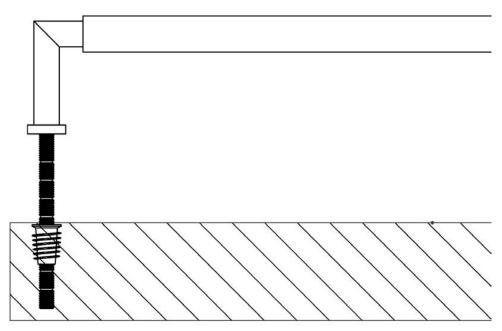
Above diagram shows how a face fix pull handle is fitted to a wooden door
