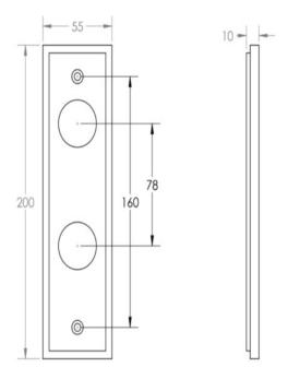
• DIN Bathroom Lever Set - 78mm Centres - (With Turn & Emergency Release)
