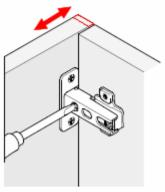
Lateral Adjustment Moving Door Left – Right
