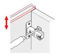
Vertical Adjustment Moving Door Up & Down
