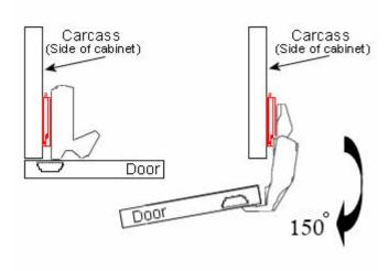
• Suitable only for doors that overlay the cabinet carcass - (see below diagram)
