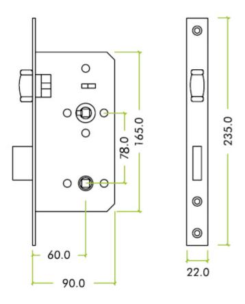
Lock Case Depth (A)Backset To Keyhole (B)Spindle To Spindle centers (C)
