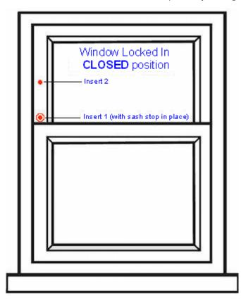
• The sliding sash window can be locked in the open position for ventilation, by screwing the sash stop into insert 2 (see below diagram)
