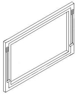
• When the fanlight window is in the open position the roller projects from the frame to restrict and support the fanlight window - SEE BELOW DIAGRAM
