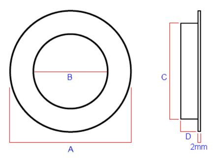
Item Code Diameter (A)Opening Diameter (B)Recess Diameter (C)Recess Depth (D)Backplate Thickness
