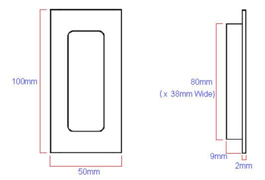
Item CodeHeightWidthRecess DepthRecess HeightRecess WidthBackplate Thickness21824.1100mm50mm9mm80mm38mm2mm
