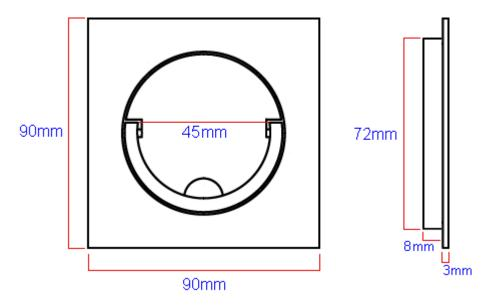
Item CodeHeightWidthRecess DepthRecess DiameterBackplate ThicknessRing Pull Size (Internal Dimension)30222.190mm90mm8mm72mm3mm45mm
