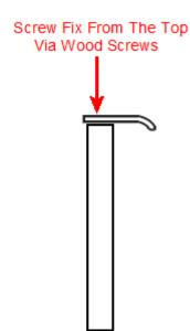
• Comes supplied with matching countersunk slotted wood screws.
