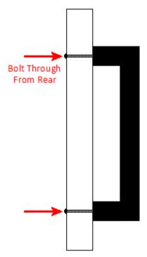
• Bolt through fixings provide a superior strong fixing allowing this handle to be fitted to tall or heavy doors.
