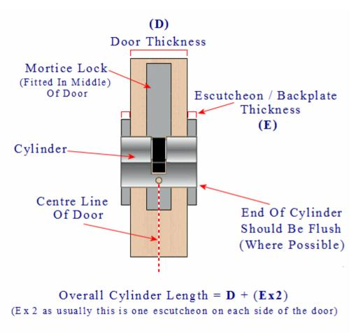
Always check the mortice lock is fitted in the middle of the door if not an offset cylinder is required
