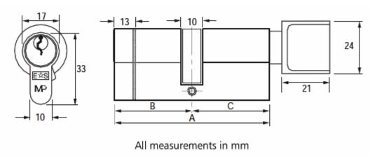
$Item\ Code\ Overall\ Length\ (A) External\ Side\ (B) Internal\ Side\ (C) Anti-Snap\ Section$
