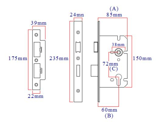
Item Code Lock Case Depth (A)Backset To Keyhole (B)Spindle To Euro centers (C)
