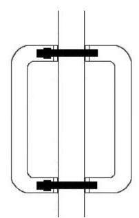
Above diagram shows how a bolt through pull handle is fitted to a wooden door
