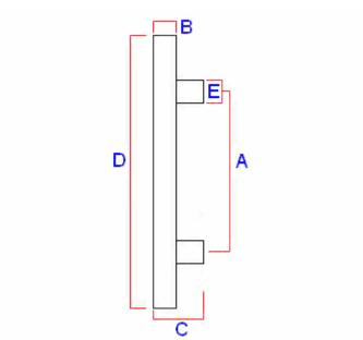
Item Bolt centers (A)Diameter (B)Projection (C)Overall Length (D)Post Diameter (E)
