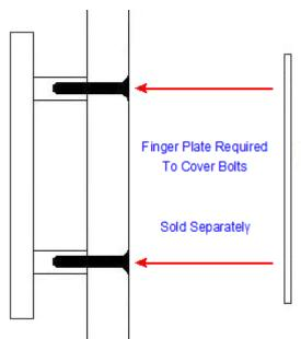
Above diagram shows how a bolt through pull handle is fitted to a wooden door
