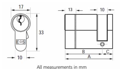
Equal cylinders for use with timber doors or doors with a mortice lock fitted in the middle of the door.
