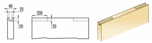
• Please note the Syntesis kit must be routered 200mm x 20mm into two positions in the top of your door, please make sure the top rail of you chosen door is deep enough to accommodate this routing.
