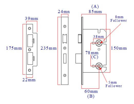
Item Code Lock Case Depth (A)Backset To Keyhole (B)Spindle To Spindle centers (C)
