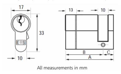
Item Code Overall Length (A)External Side (B)Internal Side (C)Anti-Snap Section
