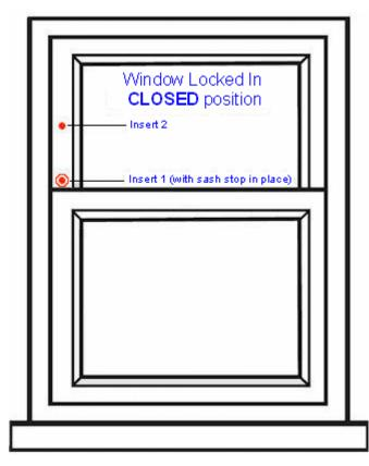
• The sliding sash window can be locked in the open position for ventilation, by screwing the sash stop into insert 2 (see below diagram)
